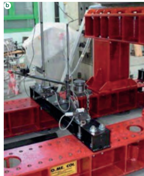
Figure 28 : Bending test: (a) test setup; and (b) measurement instrumentation (Moccichino et al. 2010).
