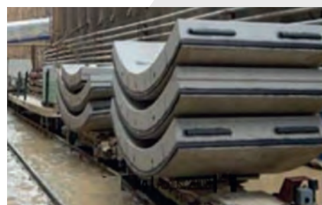
Figure 6(a) : Segments stacking for storage and transportation
