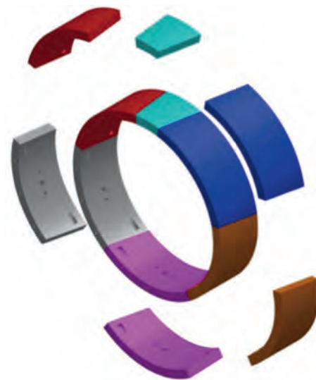
Figure 3 : Typical 6 segment ring configuration (5+1) used for tunnels 6m diameter or less
