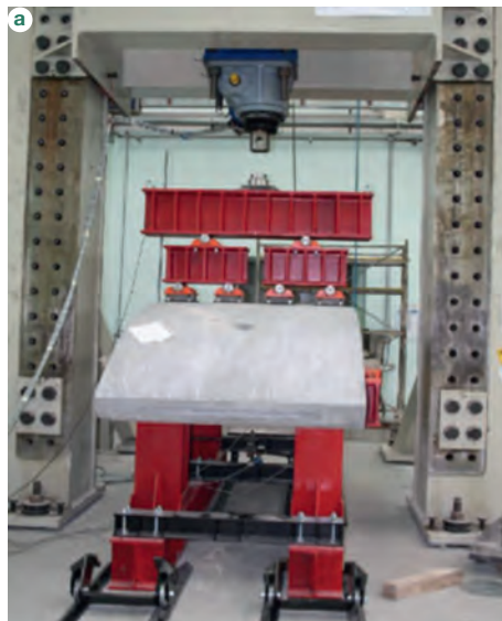
Figure 28 : Bending test: (a) test setup; and (b) measurement instrumentation (Moccichino et al. 2010).
