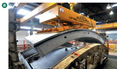
Figure 5(a) : Stripping (Demolding) segments from forms
