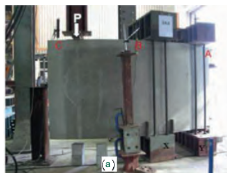
Figure 30 : Cantilever load test set-up and instrumentation (Poh et al. 2009).
