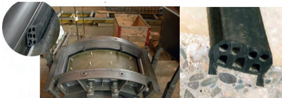
Figure 44 : Anchored gaskets fixed into the concrete segment during segment production
