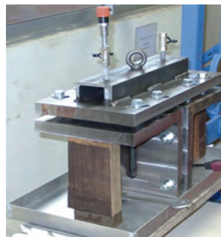
Figure 40 : T joint watertightness test setup for segment gaskets as recommended by STUVAtec (2005)
